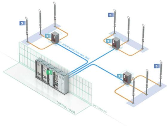
Fig. 2 Short local electrical connection of the primary sensors ③ to the RIC ② and connection of the RIC to the eLumina™ HVDC control system ① via optical fibres using the IEC 61850 protocols.
