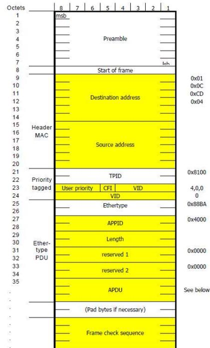
Fig. 3 Segments that can be manipulated in an SV packet.
