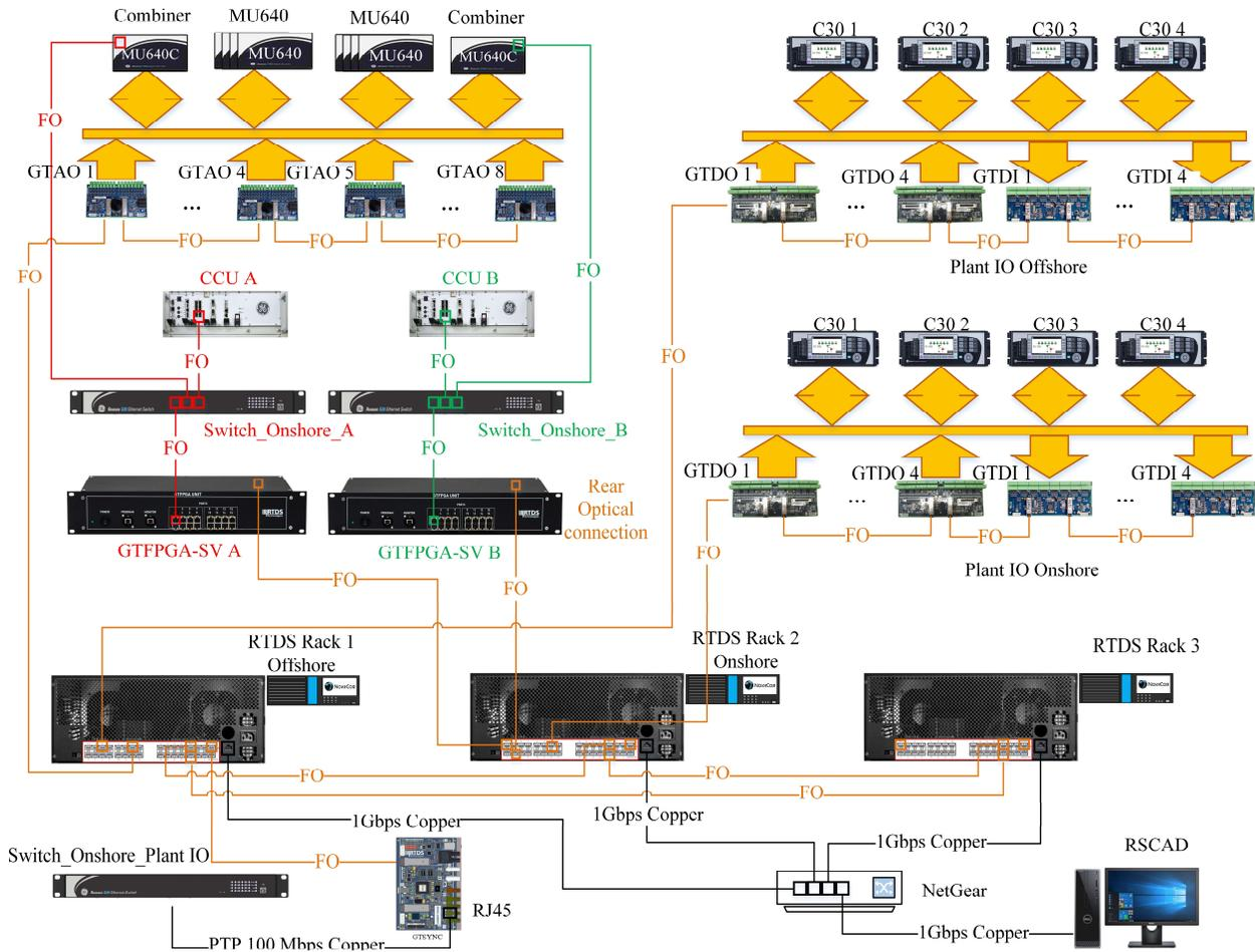
Fig. 1 Testbed for high-speed HVDC control system.
