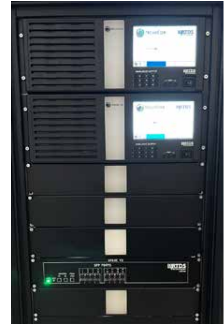
Final setup with the integration of the new GTSOC V2 in the SOFIA RTDS setup
