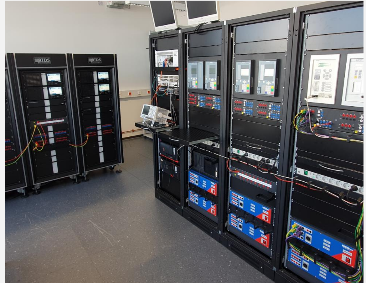
Laboratory set up at FAU for HIL
