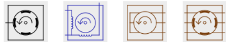
Sync Machine Permanent Magnet 1P Induction Machine Induction Machine Permanent Magnet Synchronous Machine
