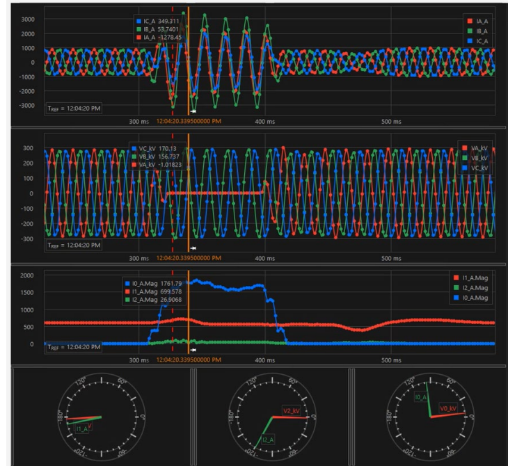
COMTRADE recording of A-G fault
