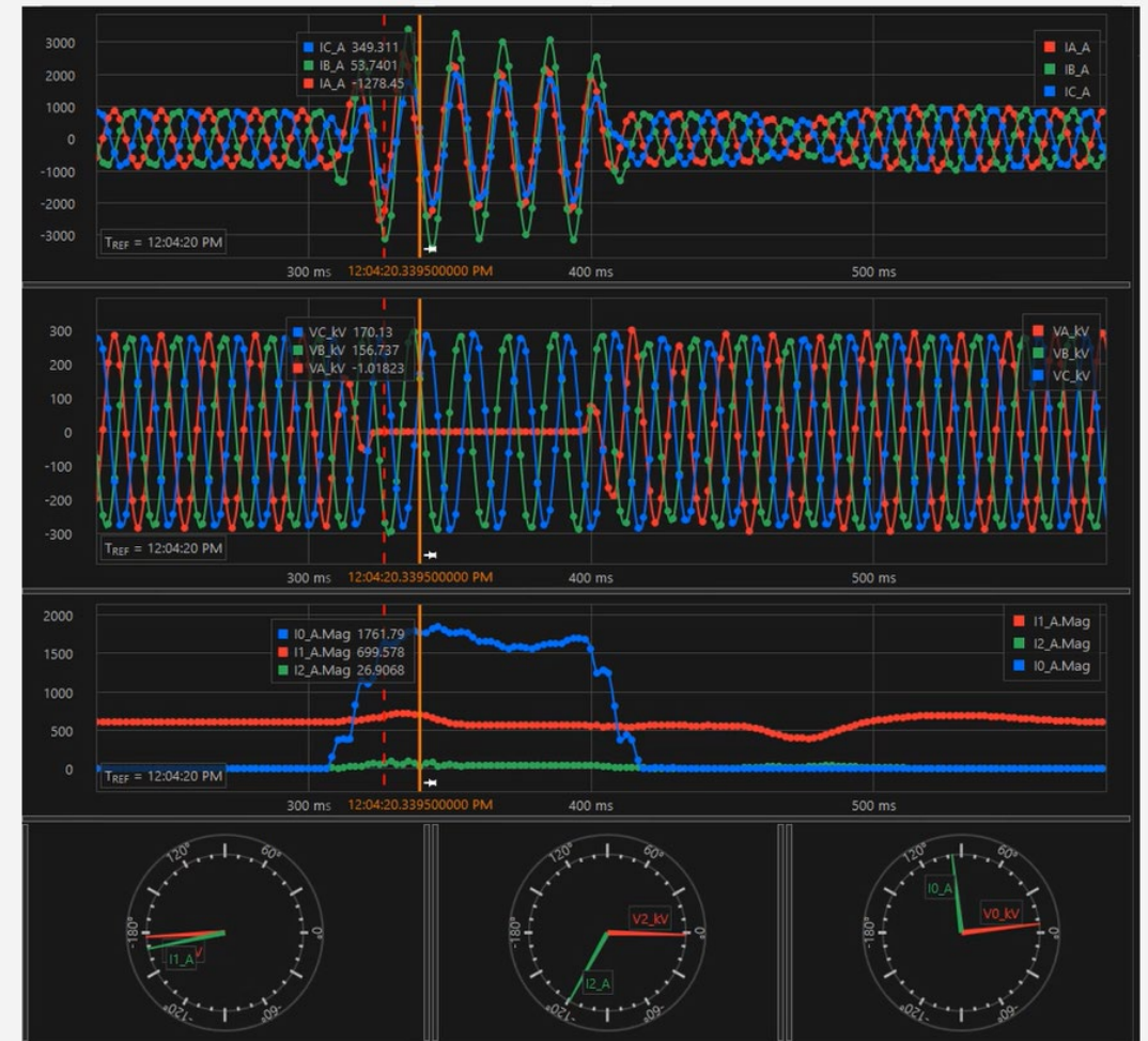
COMTRADE recording of A-G fault
