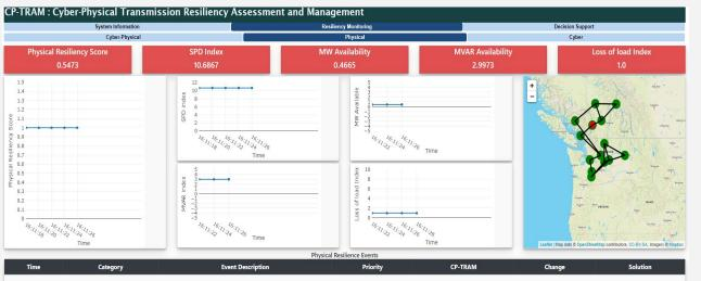
Physical Scenario, showing resiliency for Physical power system event such as tripping a breaker.
