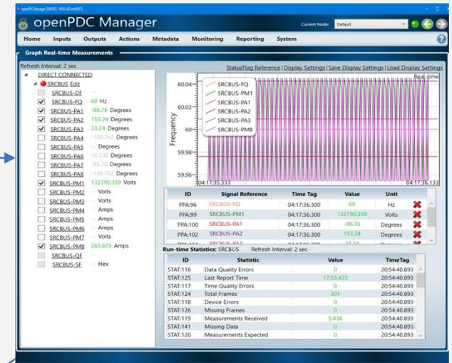
OpenPDC receiving data from substation to control center
